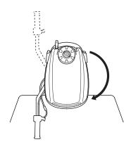
2. To reverse direction, turn the outboard motor 180°, and then pivot the tiller handle as shown. Be careful not to hold and move the throttle grip when pivoting the tiller handle.
