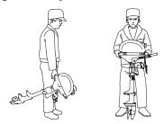
To carry the outboard motor, hold it by the carrying handle, as shown.
