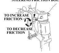
The steering friction bolt adjusts steering resistance.
