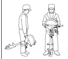
To carry, hold the outboard motor by the carrying handle, as shown.
