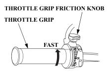
Use the throttle grip friction knob to help hold a constant throttle setting while cruising.
