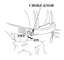
5. To start a cold engine, pull the choke knob to the ON position. To restart a warm engine, leave the choke knob in the OFF position.
