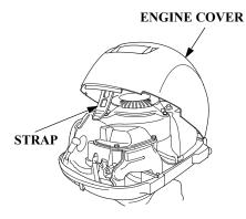
The engine cover retaining strap fastens the engine cover to the outboard motor
