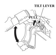
5. To return the outboard motor to the normal running position, hold the outboard motor by the front carrying handle on the engine case and pull the tilt level toward you, and then lower the outboard motor slowly.
