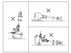
Cover the outboard motor to keep out dust. Do not use a plastic sheet as a dust cover. A nonporous cover will trap moisture, promoting rust and corrosion.
