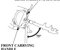
The tilt lever enables the outboard motor to be tilted for beaching, launching, or mooring.
