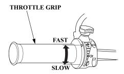
The throttle grip controls engine speed.
