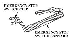
The emergency stop switch clip must be inserted in the emergency stop switch in order for the engine to start and run. The emergency stop switch lanyard must be attached securely to the operator or to the operator's PFD (Personal Flotation Device).
