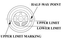
When you check the oil level in the oil level inspection window, you might notice the engine oil appears milky or the oil level has increased. If you notice either condition, change the engine oil. See the following table for an explanation of these conditions.
