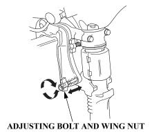
The transom angle adjusting bolt is used to adjust the angle of the outboard motor in the normal operating position (see page 34).
